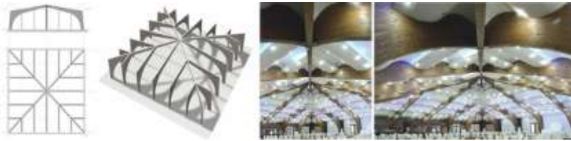
Figure 14. Large span glue laminated timber structure, Pejë
