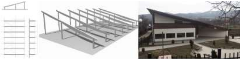
Figure 16. Glue laminated timber structure, Qabër
